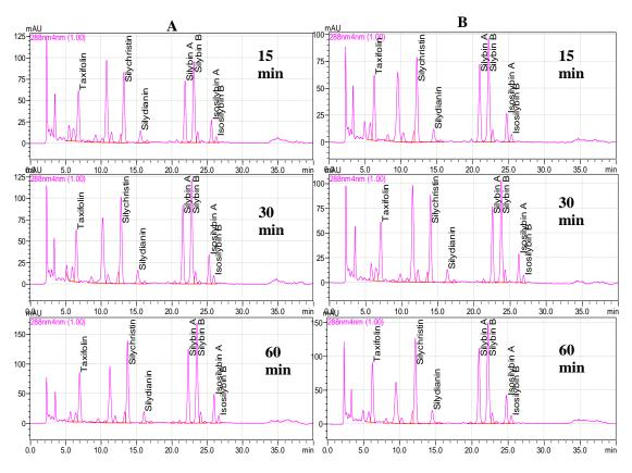
Figure 5: HPLC chromatograms of *Silybum marianum* seeds extracted using ultrasonic assisted extraction at different time intervals: [A: 20 kHz probe and B: 40 kHz bath]
